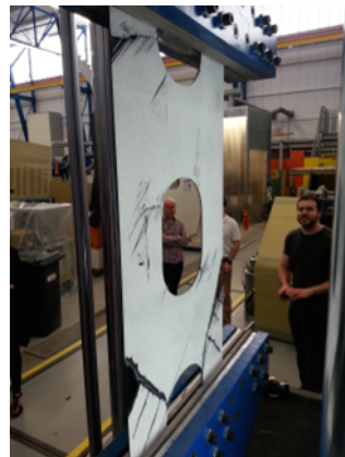
Figure 1. Failure of a variable stiffness panel loaded in tension. Note that failure is spread over the full panel instead of being concentrated at the edge of the cut-out. Courtesy Fokker Aerostructures BV, Delft University of Technology, CoDeT Engineering, NLR.
