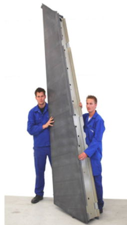
Figure 2. Induction welded thermoplastic composite business jet rudder.
