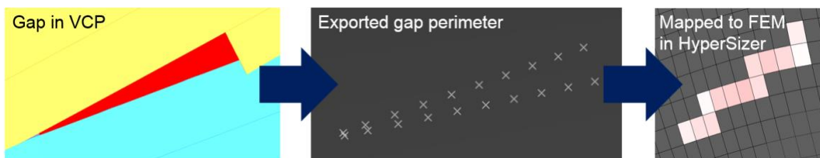
Figure 7. Lap and gap mapping approach [1].
