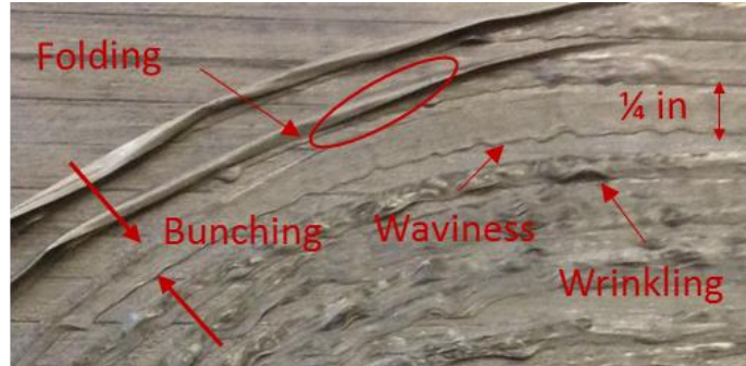
Fig. 1: Tow deformations due to excessive steering (Courtesy of McNair Center, University of South Carolina)
