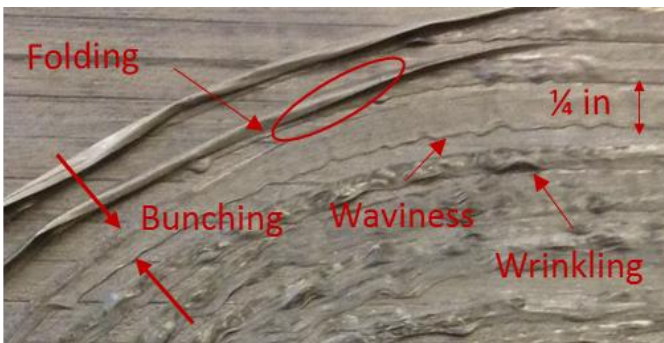
Figure 2. Tow deformations due to excessive steering (Courtesy of McNair Center, University of South Carolina) [6]
