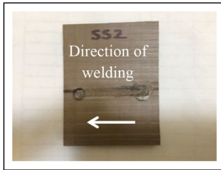
Figure 12. Specimen made using stationary shoulder.
