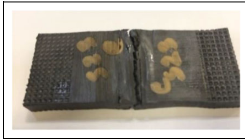
Figure 15. Generation of void lines and crack initiation.
