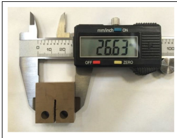
Figure 11. Compact test specimen.
