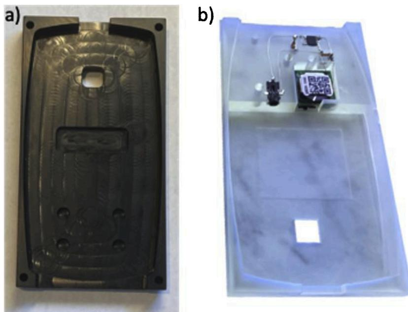
Fig. 6. Original Product (a) left), 3D printed Smart Product with Integrated Sensor System (b) right).
