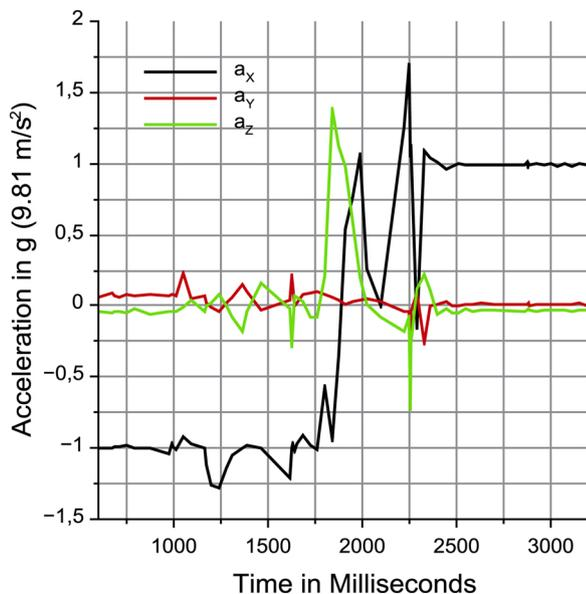
Fig. 9. Recorded Acceleration Time Series showing the Flipping Process.
