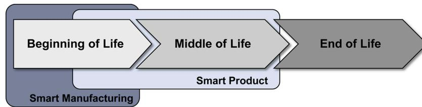
Fig. 2. Product lifecycle phases and proposed overlapping focus areas of Smart Manufacturing and Smart Products.
