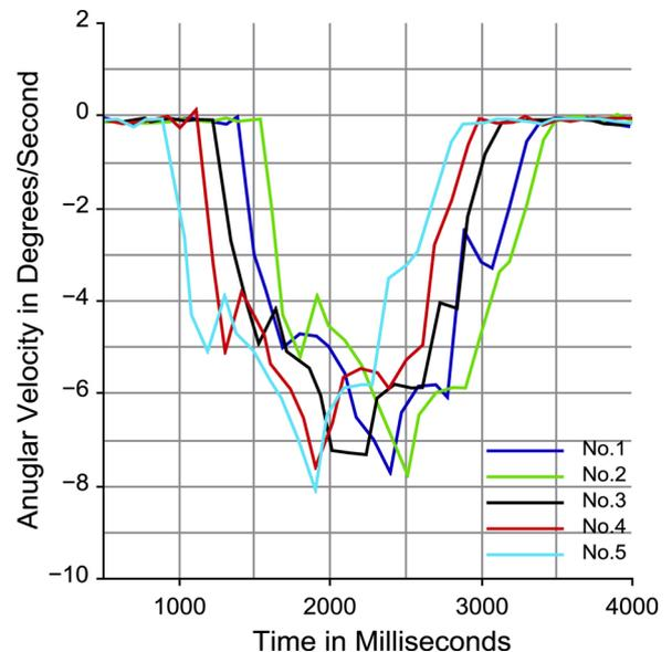
Fig. 8. Recorded Gyroscope Time Series of 90 Degrees Turn.
