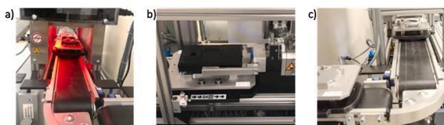
Fig. 7. a) Heat Treatment Process; b) Flipping Process; c) Right Angle Turn.
