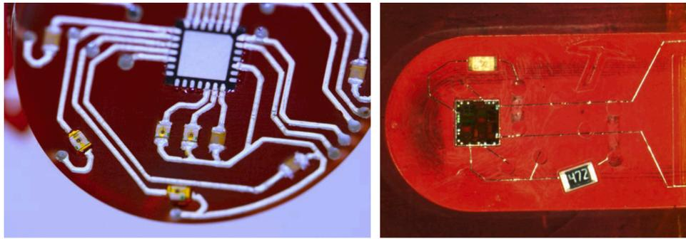
Fig. 3. Examples of 3D printed electronics: a cylindrical magnetometer (left) and a printed pill with an unpackaged silicon microcontroller and passive components (right).
