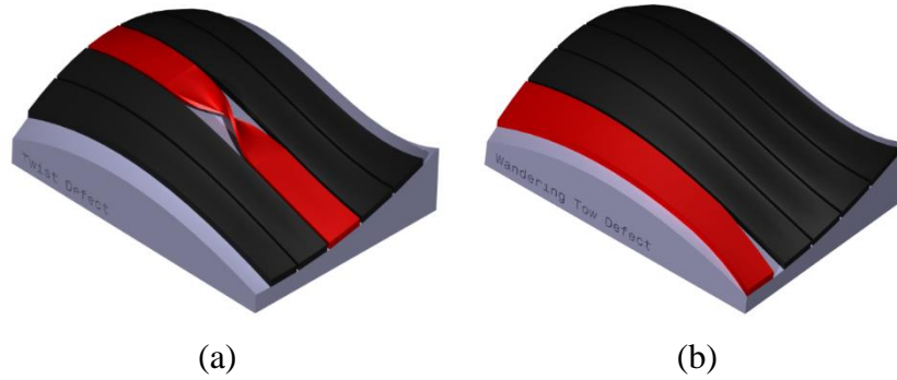
Figure 6: Example of a (a) twist and (b) angle deviation using the multiple prints method
