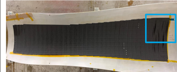
Ninety degree entire layup
