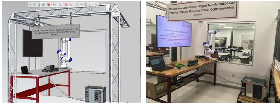
Figure 3: Stage 1 Platform. Left: virtual cell in Process Simulate. Right: physical setup.
