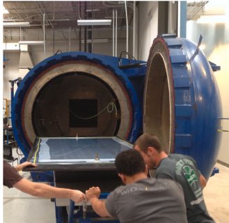
(c) Curing by Autoclave
